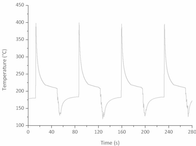
The cyclic variation of the die surface temperature generates important cyclic thermomechanical loadings, which often can end up causing cracking at the die surface in form of heat checking, corner, edge and radii cracks thermal shock cracks, especially in HPDC and squeeze casting applications. Thereby, the die cooling strategy and mechanism are also important factors that impact directly on the die durability in die casting processes.
